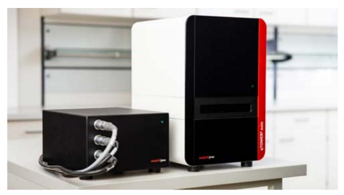
qTOWER<sup>3</sup> auto real-time PCR cycler and the power module
