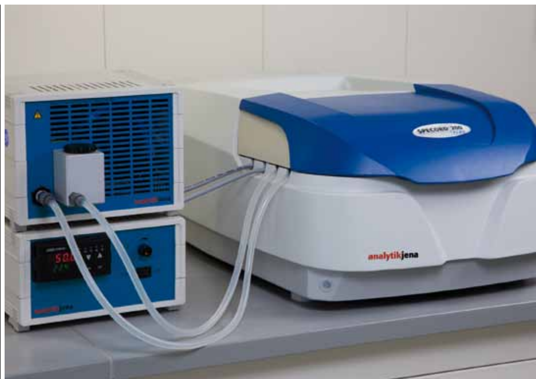
Temperature control via Peltier element
