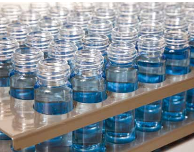
Sample rack with 64 positions for autosampler
